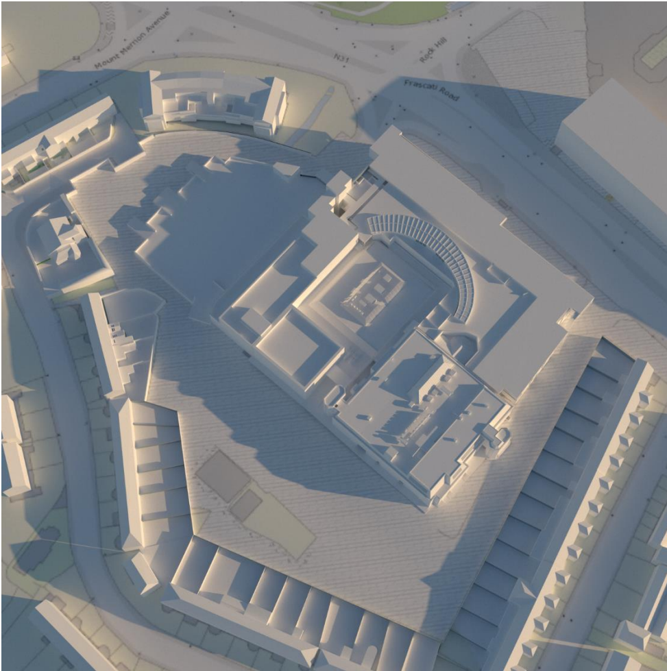
Shadows Cast at 8am (UTC+0) on the 21 st March - Before Development Scenario
