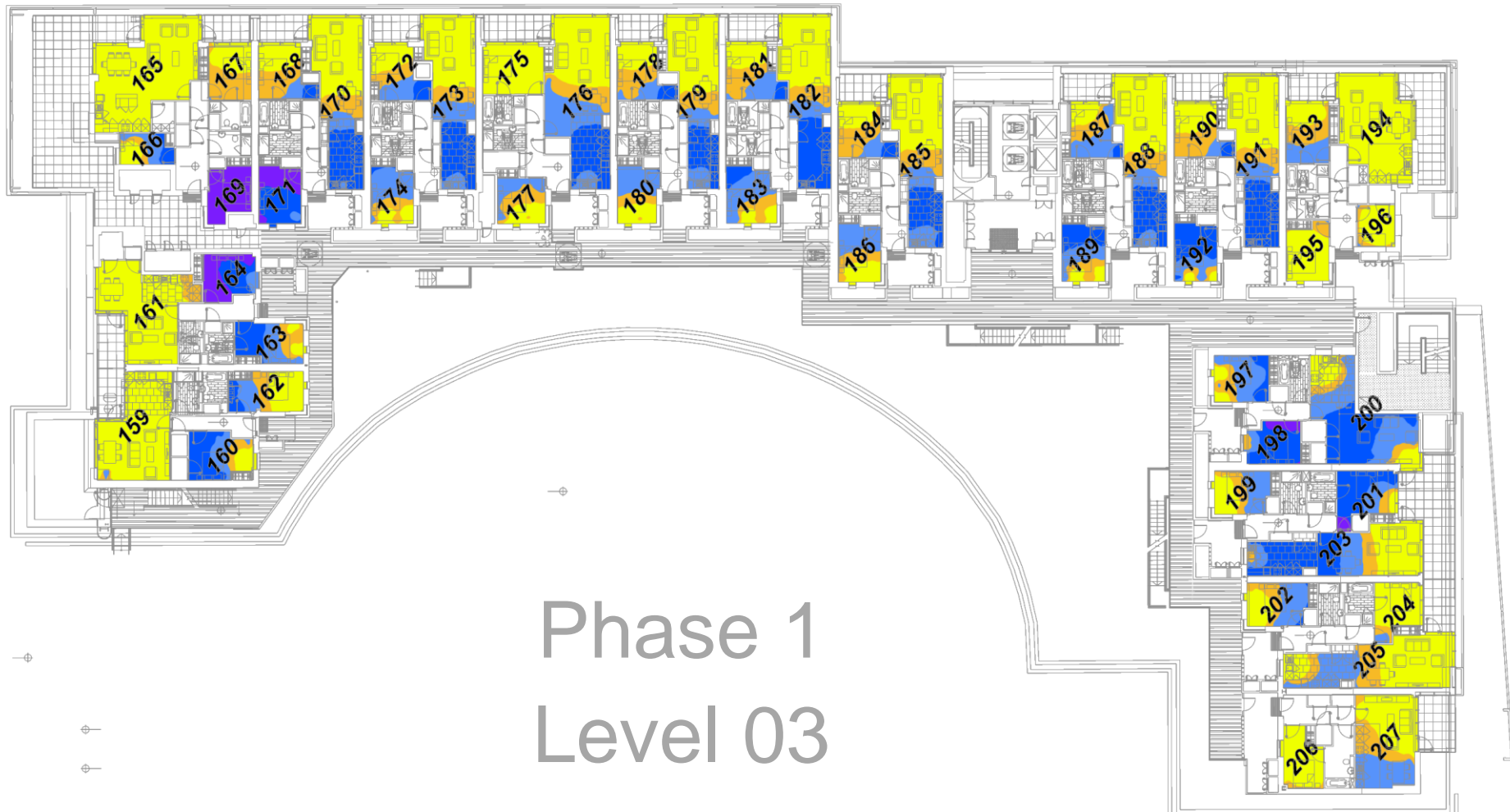
Figure 14 Daylight factor distribution diagram for rooms assessed at Level 03 in Phase 1 Development.
